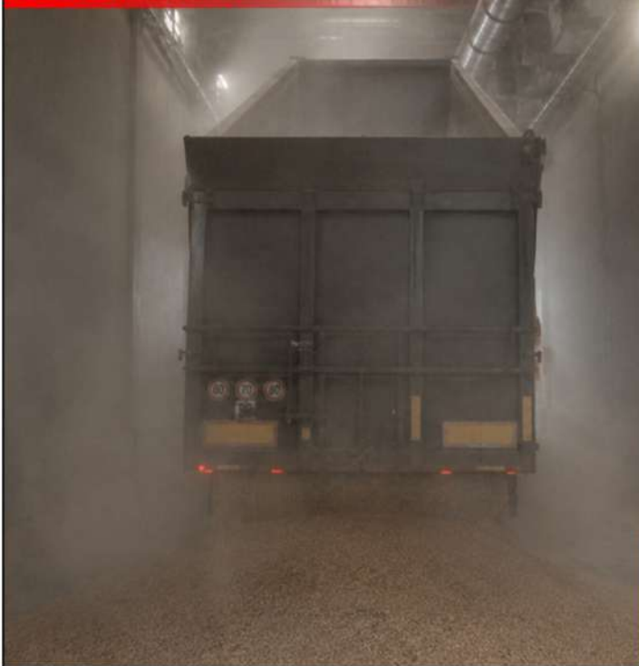
Before aspiration system installation
